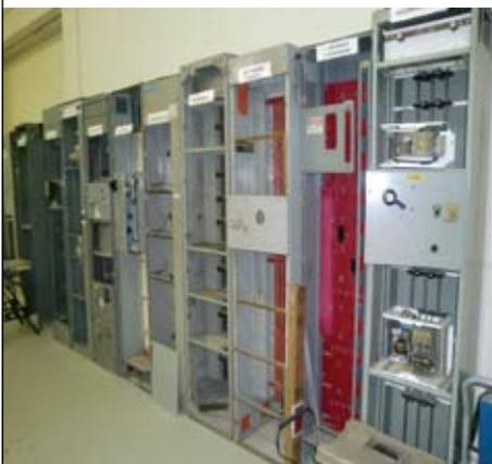
EWC has inventory of nearly every brand of MCC structures, which allows for a custom fit of each retrofitted unit.
